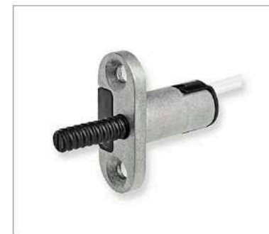
LATCH SWITCH CONTACT Installed in the keyway. Its activated through the bolt in the lock. Feedback: Door locked manually or mechanically!
