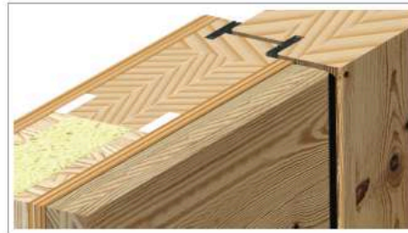
Detail: Standard-panel with strenghtening and massive-old wood application
