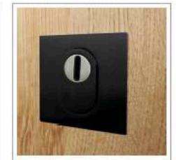
SZEP Flush – PLANO Safety rosette, rectangle shape, with cylinder cover (only 1 mm from the level of the panel) stainless steel black matt
