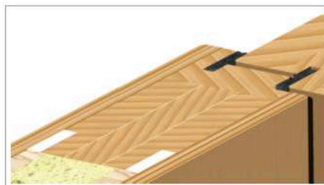
Detail: Standard-panel with strenghtening
