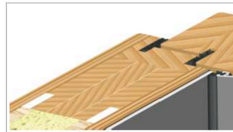
Detail: Standard-panel with strengthening
